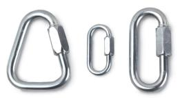
Quick Links, or also commonly known as screw links, are gaining popularity for use in situations for which carabiners are not recommended, such as when tri-axial loading cannot be avoided. The Delta shape can be used to rig anchors. The Delta can be used as a chest harness connector. While slower to open and close than a carabiner, they can be more secure when tightened down — and they cost less.
